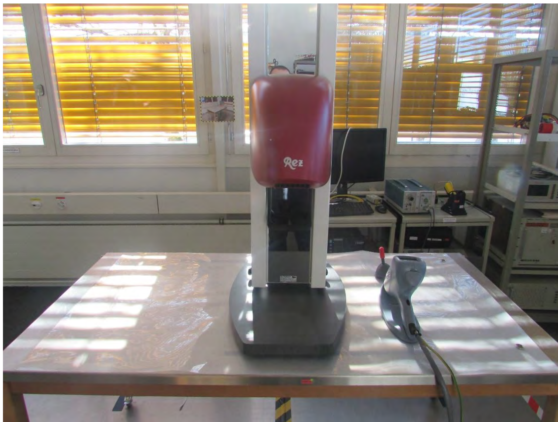
Photo 5.1.7 ..... : Electrostatic discharge immunity test (ESD) : Beluga V/S set-up
