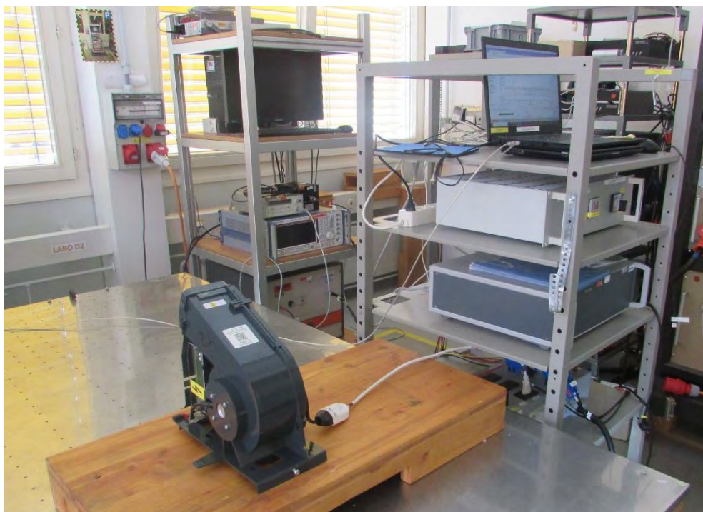
Photo 4.7.1 ..... : AC Mains Voltage fluctuation and flicker
