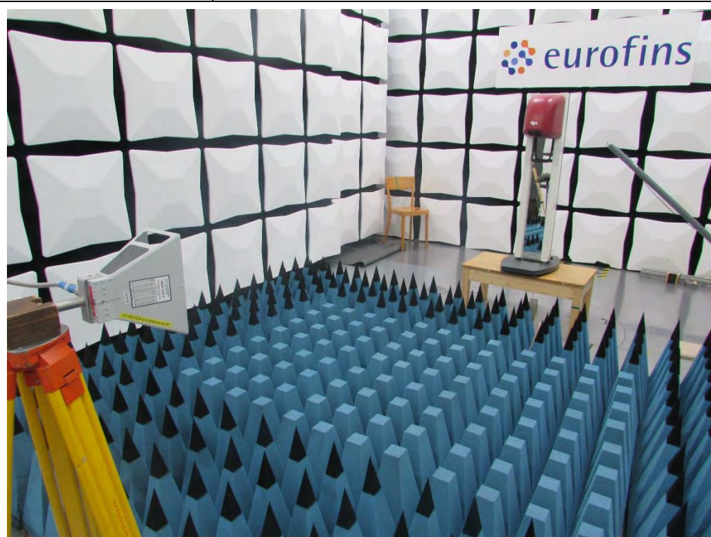
Photo 5.4.2 ..... : Radiated RF electromagnetic field immunity test : 1000 M – 6000 MHz
