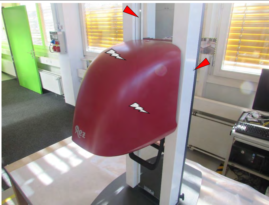
Photo 5.1.8 ..... : Electrostatic discharge immunity test (ESD) : Beluga V/S side, tests points examples
