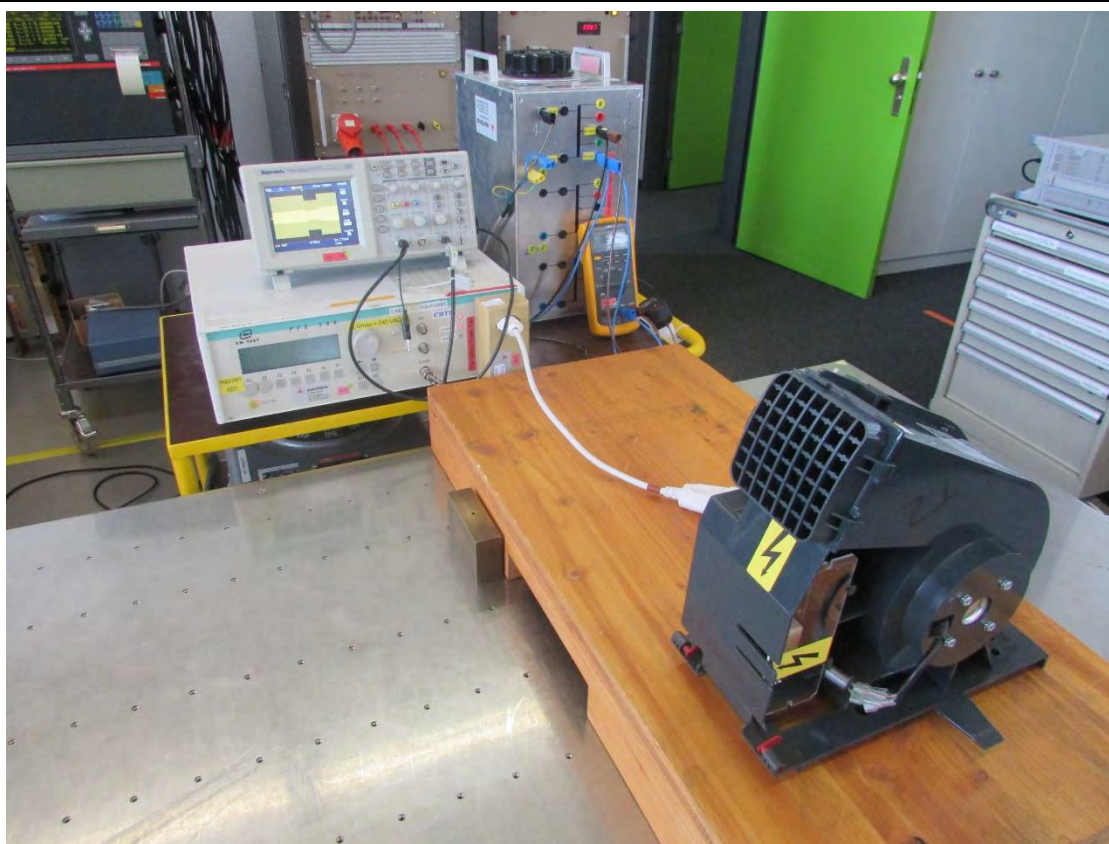
Photo 5.6.1 .....: Voltage dips, short int's and variations immunity test
